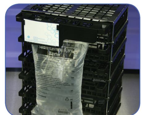
Image 3. After a Bioquell HPV bio-decontamination, the colour of the indicator portion can be used to provide an early indication of the reduction in bioburden (e.g. >6-log)
