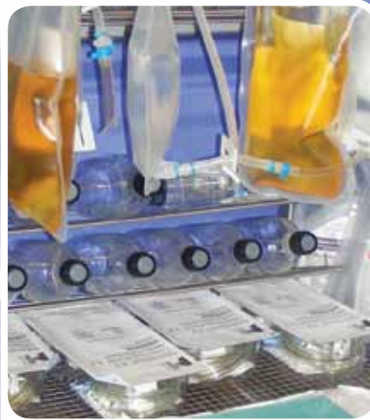
Intelligent racking ensures HPV reaches all surfaces
