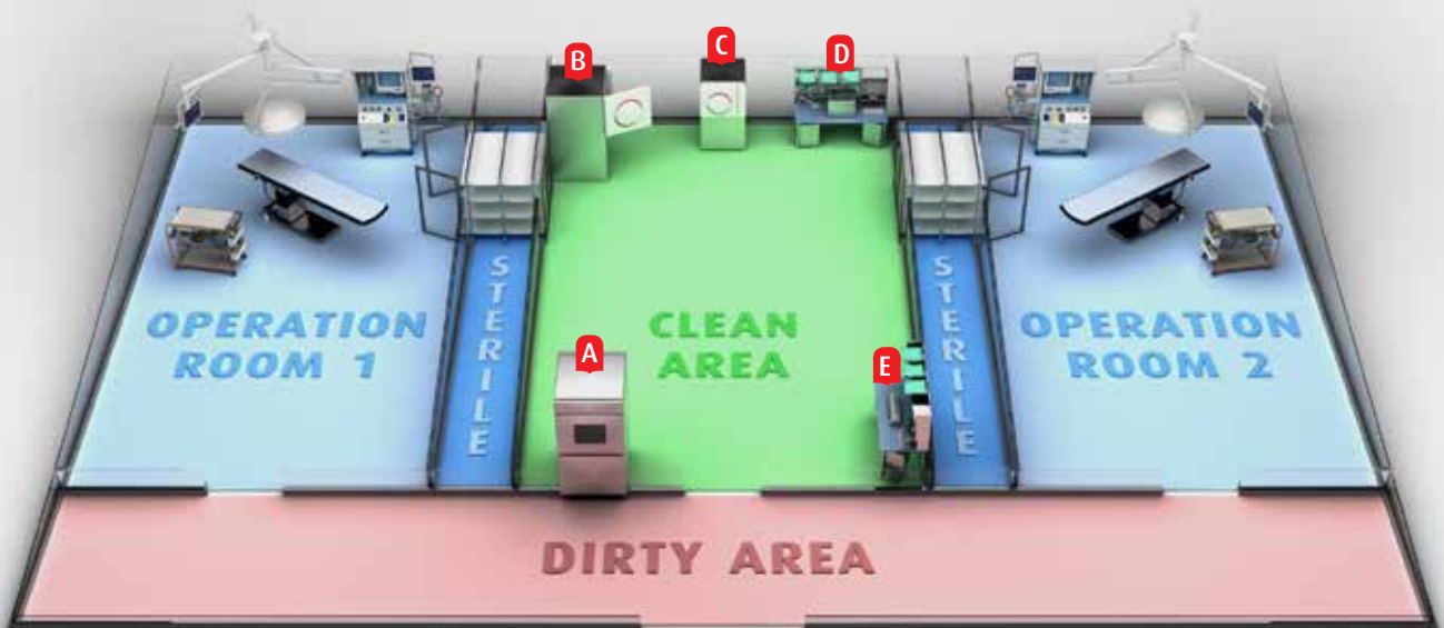
(A) Washer Disinfectator, (B) 5075HSG, (C) 3870HSG, (D) Steri-Center Packing Table, (E) Sealing Machine
